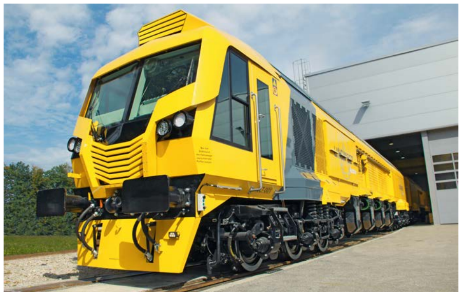
LINMAG's rail milling train MG31 at the headquarters in Steyermuehl, Austria
